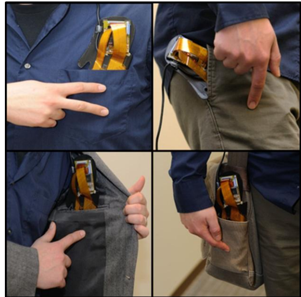
Figure 1. PocketTouch can sense multitouch finger input through a variety of garments.
