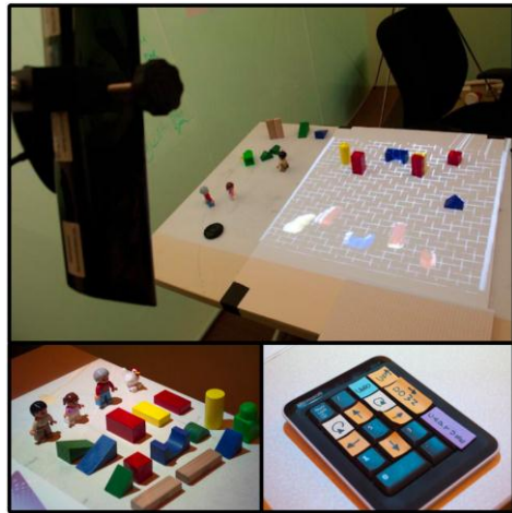
Figure 1 - Top : Workbench overview. Bottom left : Examples of physical objects available to the users. Bottom right : Wireless number pad used to manipulate the model and capture object information.
