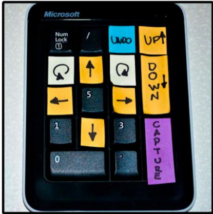
Figure 3 – Number pad used as interface device for the workbench.
