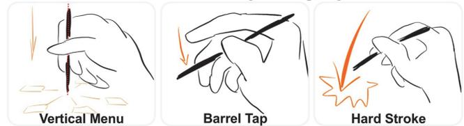
Fig. 7 A vertical posture triggers the **Vertical Menu** from the hover-state (left). **Barrel Tap** is a hard contact force perpendicular to the pen shaft (middle). **Hard Stroke** is a pen stroke that begins with a hard contact force against the screen (right).
