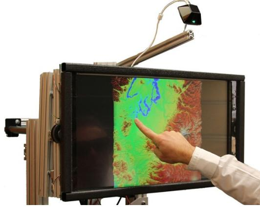
Figure 1: TouchMover 2.0 co-locates immersive 3D stereo visualization, direct touch and touch force sensing with a robotically actuated display and a vibrotactile screen.
