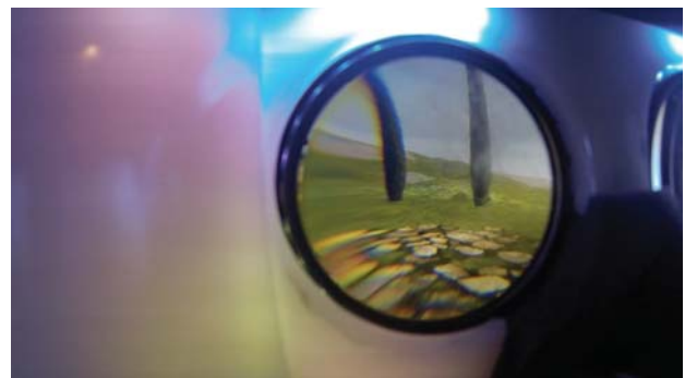
Figure 4. Close-up image from the inside of SparseLightVR. The sparse peripheral display shows the sky (top), ground (bottom), and a nearby off-screen red helicopter (left).
