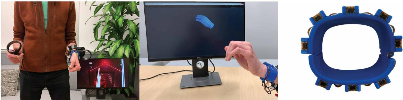
**Figure 1:** RotoWrist is a wristband that can track 2-DoF continuous relative angle of the wrist with respect to the arm. Left: A user playing Beat Saber with an Oculus Rift-S VR system. The left hand orientation is estimated using RotoWrist while a Rift-S controller tracks the right hand. Middle: Visualization of wrist angle tracking in a Unity test application. Right: RotoWrist tracking relies on eight time of flight IR modules embedded in a wristband.
